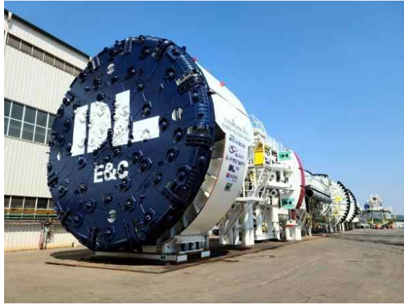
(a) TBM 조립전경
